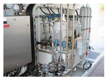
Emergency quick closing function in case of electric power supply failure HPU operated with special low temperature hydraulic fluid: AeroShell Fluid 41, intended as a hydraulic fluid in aircraft applications, for low temperatures down to -55°C.
