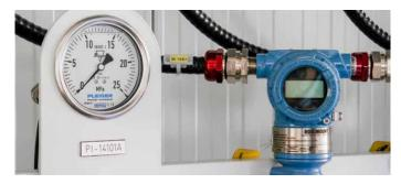
Remote control via HART-Transmitter with Ex-approval and local display. Triple instruments for oil pressure, oil level, oil temperature and air temperature. Transmitter cable and cable glands according to CSA EX-Specifications.
