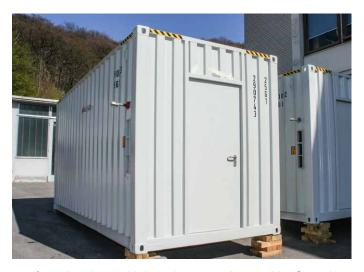
20 feet insulated high cube container with Container Safety Convention (CSC) approval as enclosure for outdoor installation and simple shipping. With space heaters, additional doors with Ex-approval and trace heated seals.
