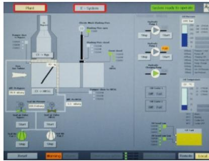
The central panel indicates the states of all HPU components on only two operating screens and thus facilitates rapid and comfortable troubleshooting – which facilitates considerably reduced downtimes in case of fault.
