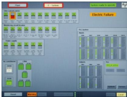
With the daylight-readable SIMATIC Multi Panel MP377 by Siemens, Pleiger Elektronik for the first time employed a central, daylight-readable operator panel instead of diverse illuminated pushbuttons. The operator is provided with more comprehensive process information in a transparent form.
